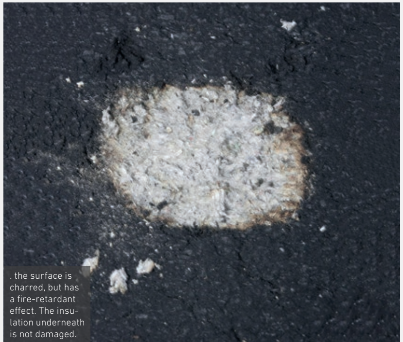
Cellulose insulation burns like wood, controlled, but safe. As a demonstration, cellulose is flame treated at 1000 °C over minutes.
