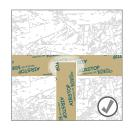
Roughen AIRSTOP SOLO Adhesive Tape below the loose end using the abrasive pad supplied. Wipe away abrasive dust. Apply pressure to attach to the matt tape below.
