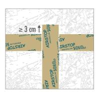
AIRSTOP SOLO Adhesive Tape can be continued  $\geq 3$  cm over the lower tape.
