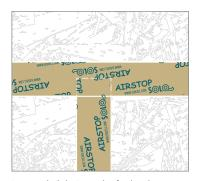
Loose end (below) can be fixed with continuous AIRSTOP SOLO Adhesive Tape.
