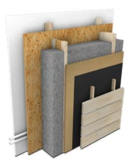
Gypsum fibreboard Installation layer (lathing e = 62,5 cm) Optional: AIRSTOP SD18 Vapour barrier OSB board (sealed airtight) Variations: structural timber or double-T beamr ISOCELL cellulose insulation Wood fibre insulating panel Wind seal (e.g. OMEGA wind seal) Rear ventilation, spruce lathing offset Larch cladding
