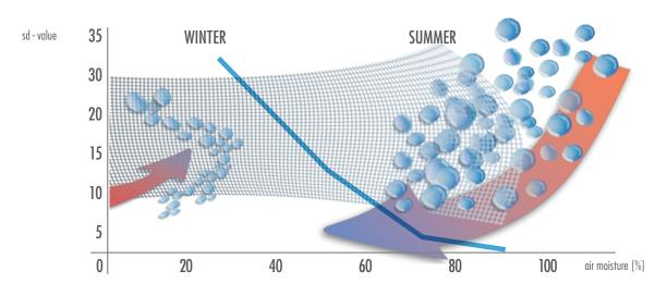
The functional membrane of AIRSTOP DIVA changes its resistance to diffusion depending on the current humidity. Usually room atmosphere is drier in the winter months. The sd-value of the moisture-variable vapour barrier increases. This process results in the penetration of only a little vapour into the construction and/or into the insulation. At 25 % relative room humidity the sd-value of AIRSTOP DIVA increases to > 30 m.
