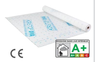
With AIRSTOP DIVA ISOCELL have developed a transparent, tear-resistant vapour barrier. The special membrane reacts to the moisture in the surrounding atmosphere. With sufficient solar insolation the moisture is transported to the interior of the construction and favourably infl uences the drying of construction components during the summer. A strong PP membrane guarantees very good stability.
